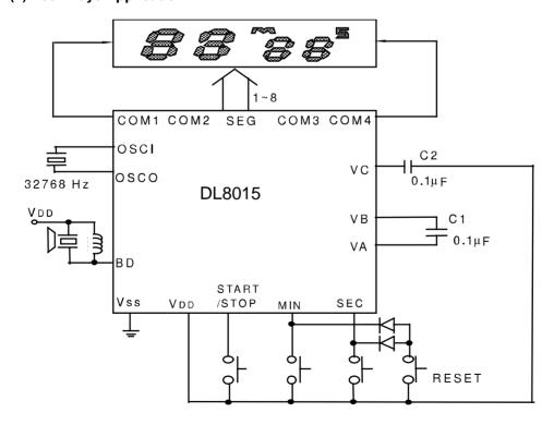
Note: Substrate must be connected to VDD.
