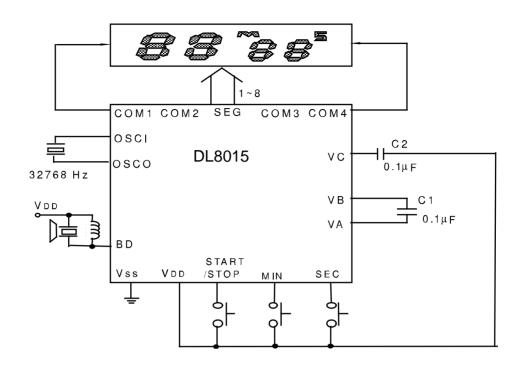
Note: Substrate must be connected to VDD.
