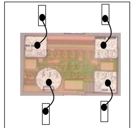
注: THE IC SUBSTRATE SHOULD BE CONNECTED TO VDD (IC衬底接正极)
