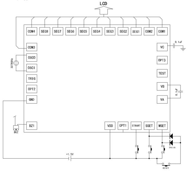
NOTE: The chip substrate must be floated or connected to VDD.
